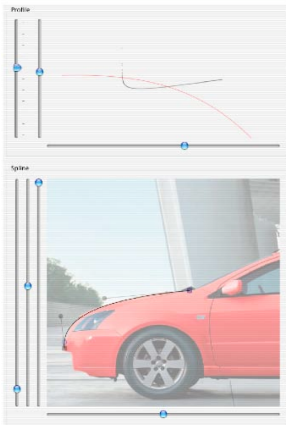
Figure 12. Car B. Impression of the shape of the nose of the car B is “convergent”. The K-vector shown above (the black bolder line) expresses that the car B has convergent curve.
