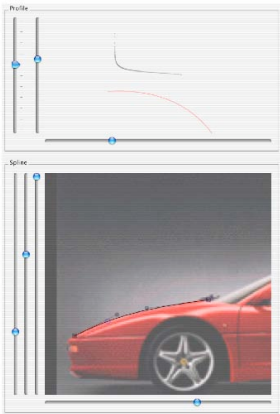
Figure 14. Car D. Impression of the shape of the nose of the car D is “divergent”. The K-vector shown above (the black bolder line) expresses that the car D has divergent curve.
